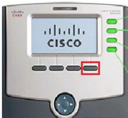
*Figure 1: the red highlighted key is the “xfer” option during a call.*
